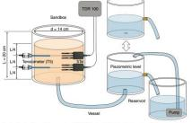
Fig. 1. Design of the sandbox experiment. The TDR probes (CS640) and tensiometers (T5) were placed at the locations 15 and 10 cm from the top of the sandbox. The water injection and draining tube was at the bottom of the sandbox and connected to a reservoir. A vessel was used to collect the water released from the reservoir.
