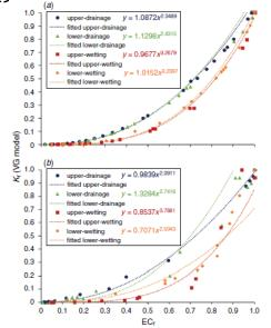
Fig. 5. The power law relationships between  $EC_{\tau}$  and  $K_{\tau}$  of (a) Quartz sand and (b) Ottawa sand based on VG model.
