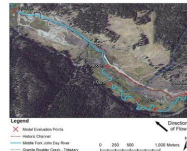
RE 2 Aerial imagery of the Middle Fork of the John Day River on the Oxbow Conservation site. The labelled locations correspond to of comparison between the model and monitored data and other points of analysis. Restoration led to the closure of the river channel and with red dashes, and extended the tributary (dark blue) into the south channel [Colour figure can be viewed at wileyonlinelibrary.com]
