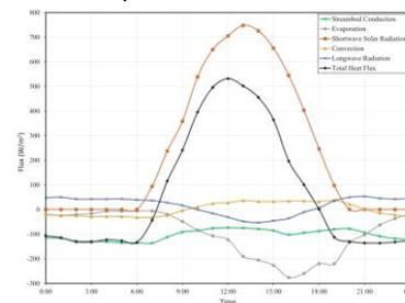
FIGURE 6 Modeled energy fluxes for an unshaded section of the MFJDR encompassed by the Phase 2 project for August 6. Shortwave solar radiation controls the energy budget and is the primary driver for stream heating [Colour figure can be viewed at wileyonlinelibrary.com]
