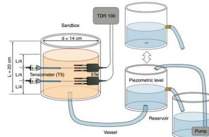
Fig. 1. Design of the sandbox experiment. The TDR probes (CS640) and tensiometers (T5) were placed at the locations 15 and 10 cm from the top of the sandbox. The water injection and draining tube was at the bottom of the sandbox and connected to a reservoir. A vessel was used to collect the water released from the reservoir.
