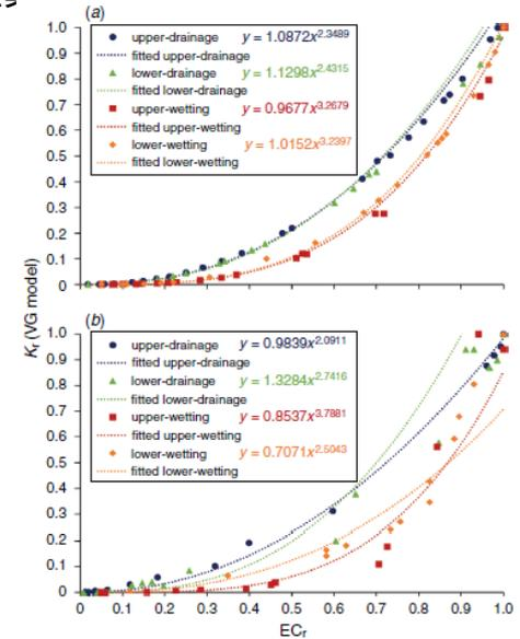
Fig. 5. The power law relationships between  $EC_r$  and  $K_r$  of (a) Quartz sand and (b) Ottawa sand based on VG model.
